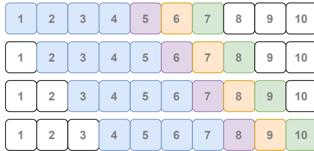
Fig. 4. Illustration of the sliding window technique for a sample of 10 timesteps, where each number denotes a distinct time step. As an example here, the input horizon (blue color) length is 4 timesteps and the output horizon length is 3 timesteps. The input window slides 1 time step at a time across the entire data sequence to generate 4 distinct input and forecast horizon pairs. The purple, orange, and green colors of the output horizon represent 1-day, 2-day, and 3-day ahead forecasting, respectively. The timesteps of 1-day ahead forecasting across the data sequences are then concatenated into a single timeseries list that is called 1-day ahead prediction. The same for 2-day and 3-day ahead.
